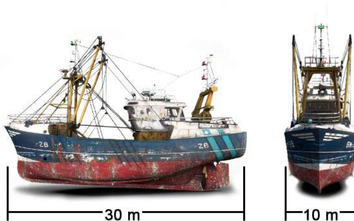
Figure 4.29: Illustration of the dimensions of a typical 1000GT vessel used for the shadowing analysis
